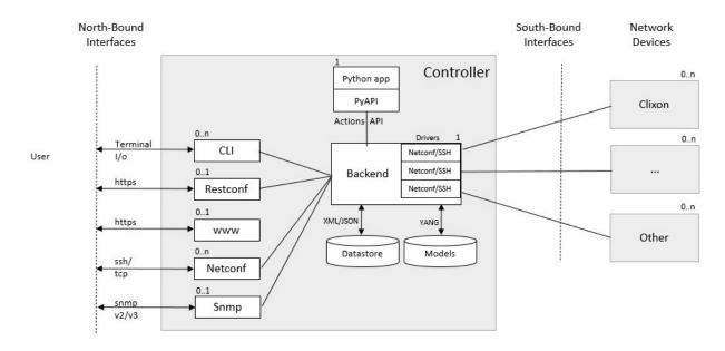
The controller is built on the base of the CLIgen/Clixon system, where the controller semantics is implemented using plugins. The *backend* is the core of the system controlling the datastores and accessing the YANG models.
